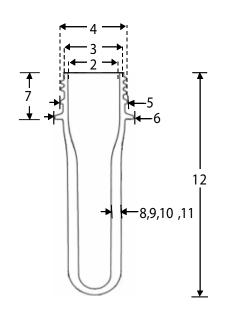
NOTE: THICKNESS 1, 2, 3 AND 4 ARE  $90^{\circ}$  EACH OTHER. HEIGHT FROM SUPPORT LEDGE = HEIGHT OF FINISH
